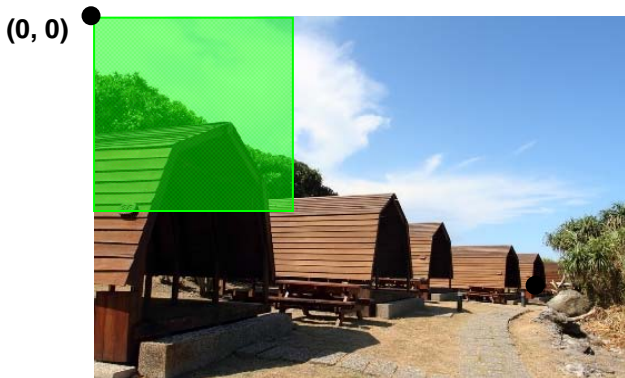
Figure 4-51 : Source0 is Layer1[(0,0) ~ (199,199)] ,Source1 is Layer2[(0,0) ~ (199,199)], executes alpha blending and showing on Destination Layer1[(0,0) ~ (199,199)], alpha = 16.
